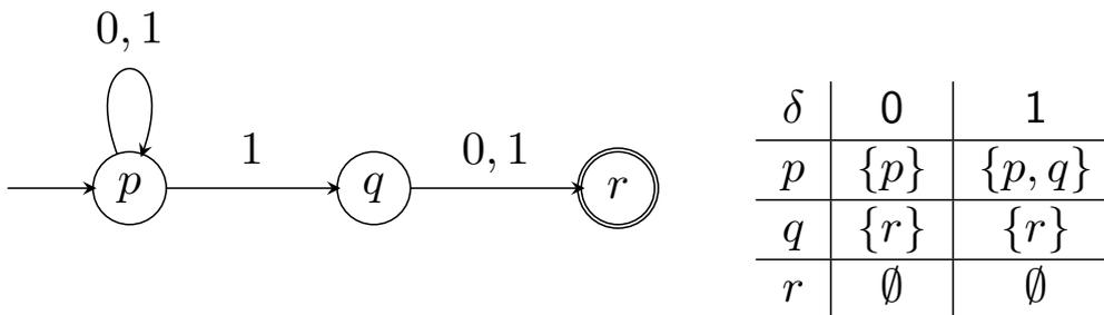
Alternative: Relation  $\delta \subseteq Q \times \Sigma \times Q$
