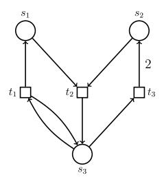
Let  $M_0 = (0, 1, 0)$  and M = (1, 0, 1). We wish to determine whether M is coverable from  $M_0$ . After one iteration of the backward reachability algorithm, we obtain the minimal basis  $X = \{(2, 1, 0), (0, 0, 1)\}$ .
