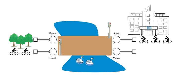
Model the bridge as a Petri net (with weighted arcs) by extending the partial model shown above. Cyclists should flow from  $p_{\text{wait}}$  to  $p_{\text{leave}}$ , and from  $q_{\text{wait}}$  to  $q_{\text{leave}}$ . Assume that, initially, the left green light is on, the right red light is on, and the bridge is empty. Make sure that the model respects safety, i.e. that bikes are not allowed to go in opposite directions simultaneously, and that the bridge cannot hold more than six bikes.
