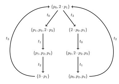
(b) It is 3-bounded since all markings of the reachability graph have at most three tokens in each place. It is deadlock-free since every marking of the reachability graph has an outgoing arc. It is live because for every transition t, every marking M of the reachability graph leads to a marking M' with an outgoing arc labeled by t.
