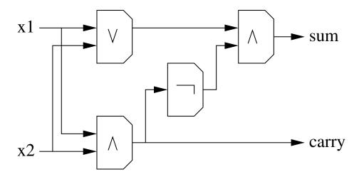
The circuit has got two inputs  $(x_1, x_2)$  and two outputs (carry, sum). Their admissible combinations can be denoted by Boolean 4-tuples, e.g. (1, 0, 0, 1)  $(x_1 = 1, x_2 = 0, carry = 0, sum = 1)$  is a possible combination.
