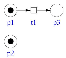
The BDD  $F_{t_1}$  describes the effect of  $t_1$ , where  $p_1, p_2, p_3$  describe the state before and  $p'_1, p'_2, p'_3$  the state after firing  $t_1$ .
