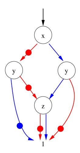
The red arc leaving the z-labelled node has its negation bit set, it therefore effectively leads to 0.
