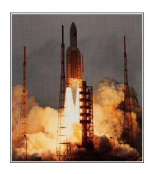
Ariane 5 began to disintegrate 39 seconds after launch because of aerodynamic loads resulting from an angle of attack of more than 20 degrees.
