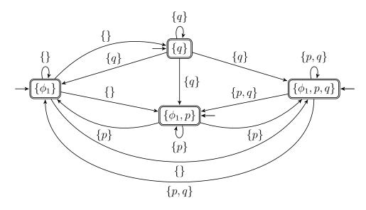
(d) Notice that  $\neg \phi \equiv \mathbf{F} \mathbf{G}(\neg p \lor (\neg p \mathbf{R} (p \lor \neg q)))$ . It suffices to add a self-looping initial state and transitions from it to all states in (c).
