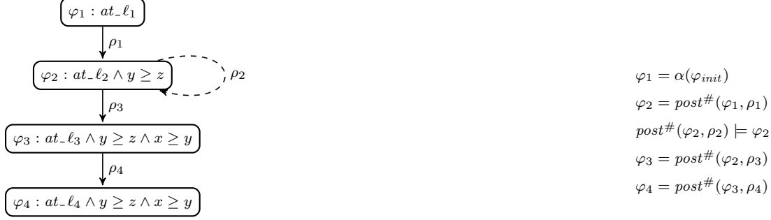
Fig. 0.3 Applying ABSTREACH on the program in Figure 0.1 and the set of predicates Preds = \{false, at\_l_1, \dots, at\_l_5, y \geq z, x \geq y\} . The nodes \varphi_1, \dots, \varphi_4 represent elements of ReachStates^\# . Labeled edges connecting the nodes represent Parent . The dotted edge denotes the entailment relation between post^\#(\varphi_2, \rho_2) and \varphi_2 .
