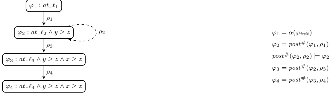
Fig. 0.10 Applying ABSTREACH on the program in Figure 0.1 and the set of predicates Preds = \{false, at\_l_1, \dots, at\_l_5, y \geq z, x \geq z\} .
