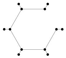
The coordinates of the inner nodes are  $R \cdot (\cos \frac{k \cdot 2\pi}{n}, \sin \frac{k \cdot 2\pi}{n})$ , for the outer nodes  $(R + c) \cdot (\cos \frac{k \cdot 2\pi}{n}, \sin \frac{k \cdot 2\pi}{n})$  where  $n = 6, k = 1, 2, \ldots, 6, R = 2cm, c = 0.5cm$ . Distances are given by the Euclidean norm if there is an edge, otherwise  $\infty$ .
