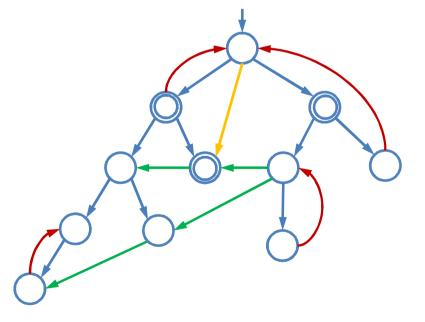
Invariant of *OneStack*: The repeat loop cannot remove a grey root  $\rho$  from the stack (remove = pop and don't push back), and can only pop states *s* such that  $d[s] \ge d[\rho]$ .
