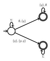
(c) Note that  $p \wedge \neg (\mathbf{XF}p) \equiv p \wedge \mathbf{XG} \neg p$ . We construct a Büchi automaton for  $p \wedge \mathbf{XG} \neg p$ :
