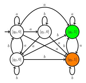
The resulting generalized Büchi automaton is the union of A and B. Note that A is essentially already a standard Büchi automaton, it suffices to make state  $[q_1, 1]$  accepting. However, it remains to convert B into a standard Büchi automaton B':
