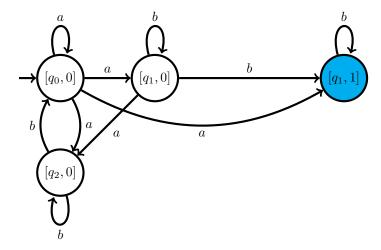
Automaton B is as follows with acceptance condition  $\{\{q_0\}, \{q_2\}\}$ :
