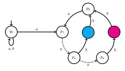
$B_{m,n}$  accepts  $L_{m,n}$  when taking the acceptance condition  $\{(\{r\}, \{s\}), (\{s\}, \{r\})\}$ . Moreover,  $B_{m,n}$  has  $\max(m, n) + 3$  states.
