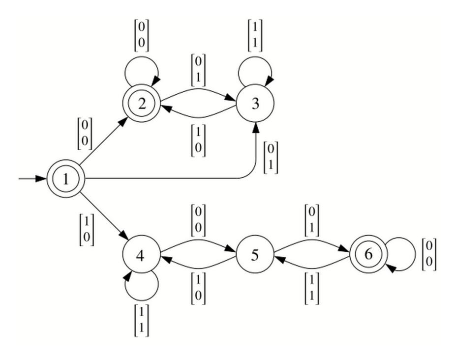
**Definition 5.3** A transducer over  $\Sigma$  is an NFA over the alphabet  $\Sigma \times \Sigma$ .
