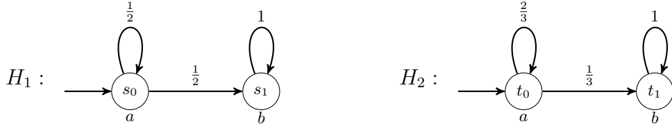
Figure 2: Two HMCs. Here H_1 and H_2 are not distinguishable but not equivalent.
